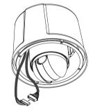
8. Fix the external cover to the housing using four screws.
